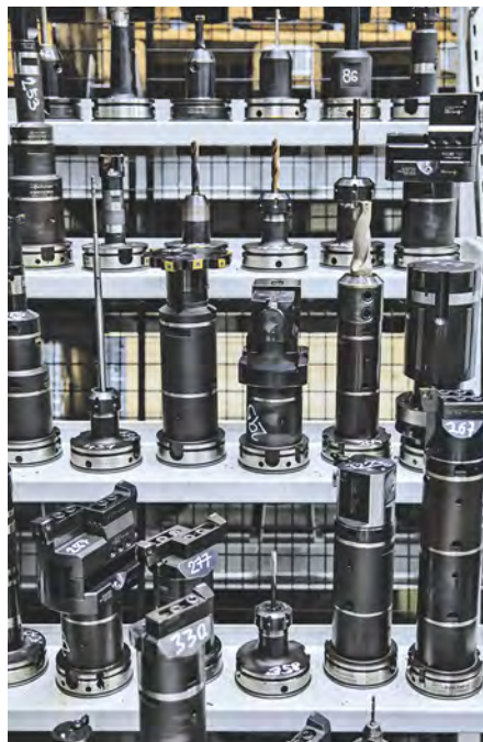
The tool changer of the machining center holds about 200 tools, and another contains an external magazine (Image r.)
