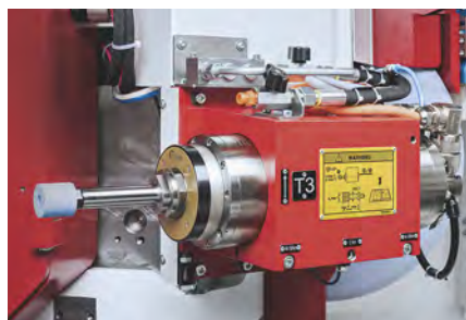
The internal grinding unit of the STUDER S33
