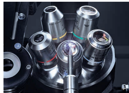
The microscopic optics of the HELICHECK NANO allow measurements in the nano range
